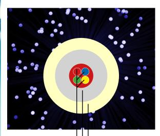
Optical fibre: 4 single-mode G657 fibres with low bend radius, under easy strippable thermoplastic skin Outer sheath: Sheath zero halogen, flame retard (LSOH), UV stabilised Ivory, compliant EN 50290-2-27
